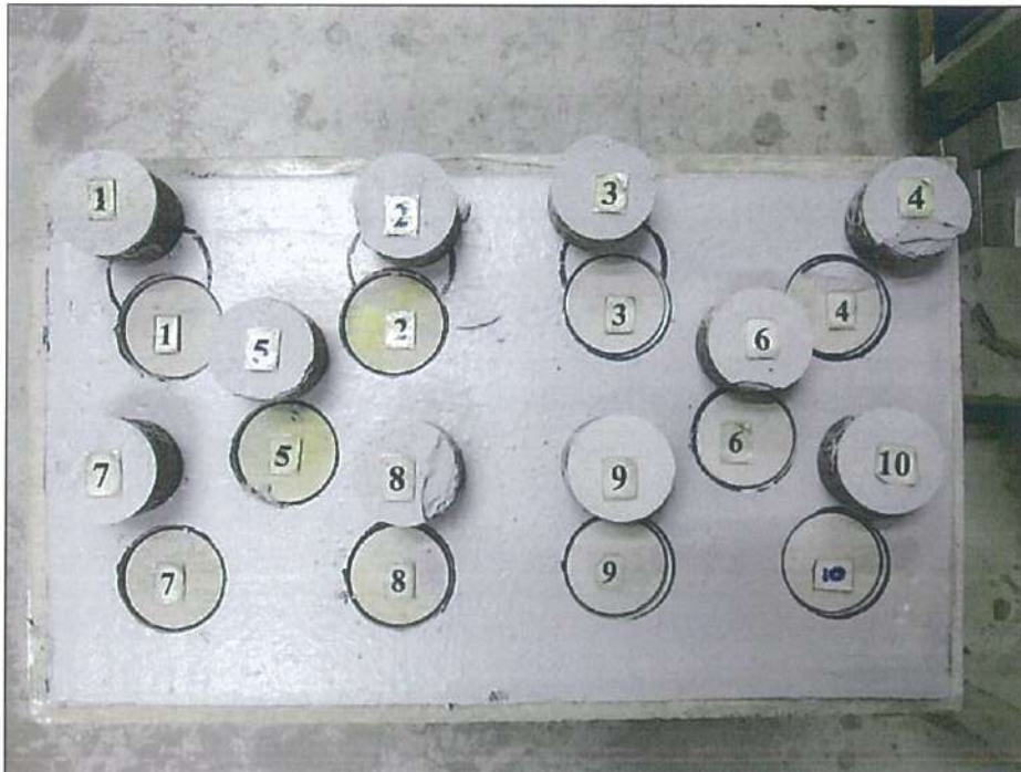
Photograph 1: shows tensile adhesion strength test at age of 14 days.
