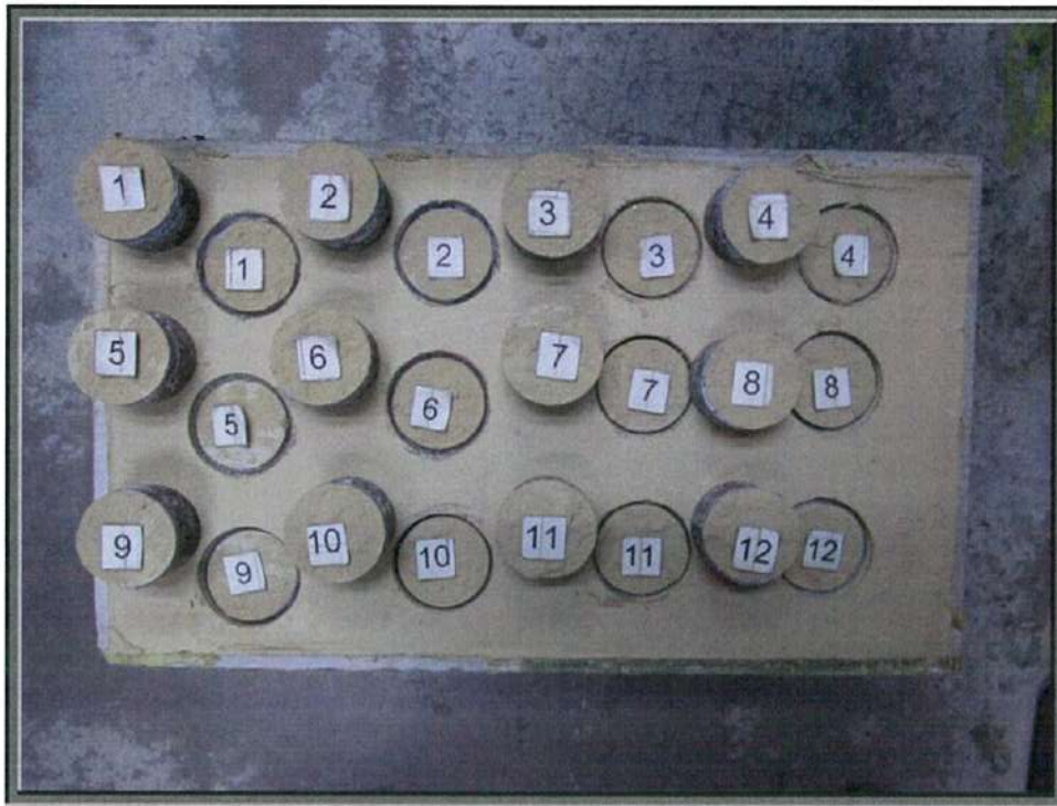
Photograph 3: shows tensile adhesion strength test after accelerated weathering.
